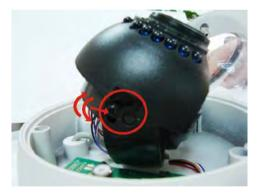
6. Screws for changing the angle of the lens
